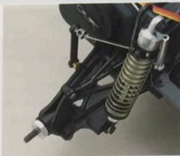
DOUBLE WISHBONE REAR SUSPENSION WITH PLATINUM OIL-FILLED SHOCKS AND STABILIZER BAR. LONG SUSPENSION TRAVEL.
