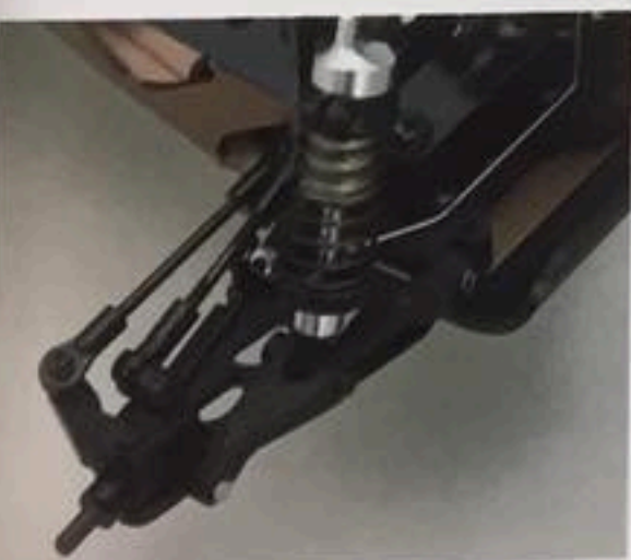
DOUBLE WISHBONE FRONT SUSPENSION WITH PLATINUM OIL-FILLED SHOCKS AND STABILIZER BAR. STRONG NYLON PARTS.
